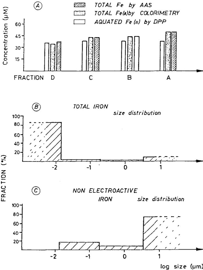
**Figure 8** (A) Analytical data obtained from an *in situ* ultrafiltration within the hypolimnion of Lake Bret at 13.5 meters depth on the 2nd of October 1985. Nuclepore filters with a nominal pore size of 3 and  $0.2 \mu\text{m}$  and an Amicon XM 300 with a molecular cut-off of 300,000 were used in this experiment. (B) and (C) size distributions for total and non electroactive iron, respectively computed from this data.
