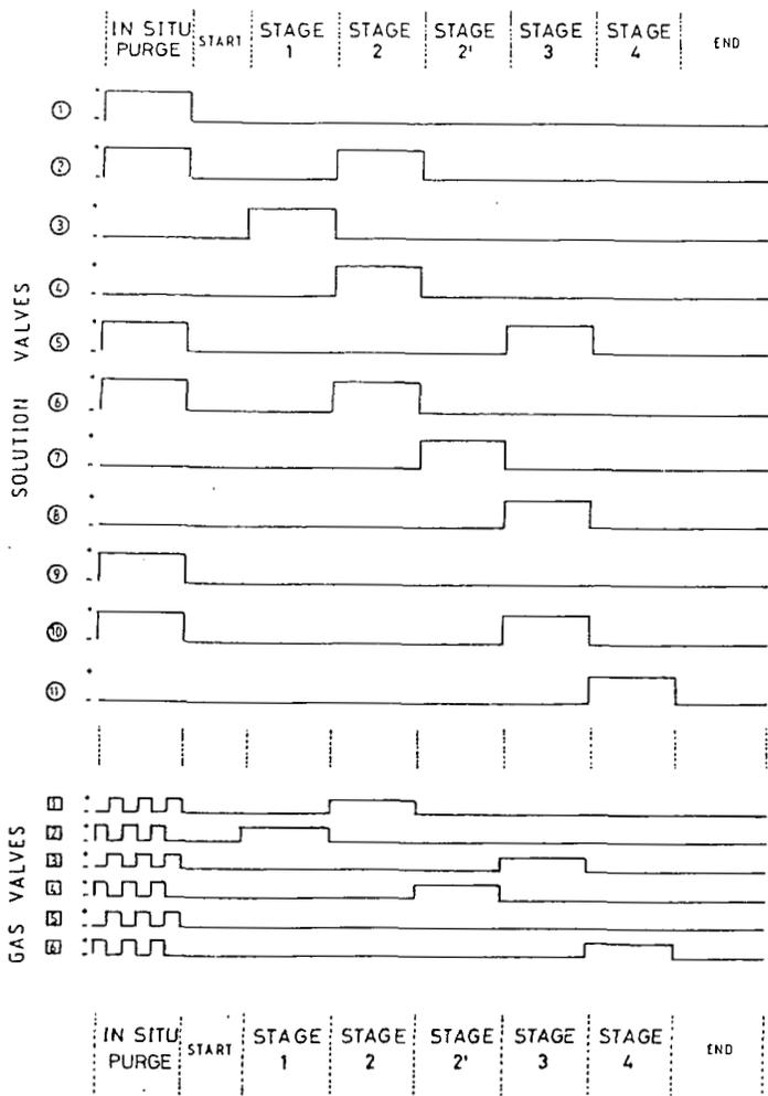
**Figure 4** Status of the eleven solution valves and the six gas valves during the eight different steps performed during an ultrafiltration.
