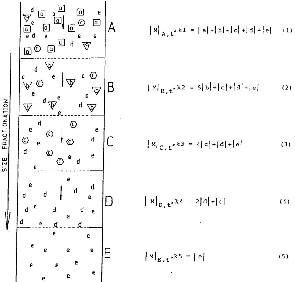
**Figure 5** Schematic representation of the mode of size fractionation used to fractionate particles *in situ*. Equations 1–5 enable calculation of the concentration of particles in a given size fraction defined by the filters used.
