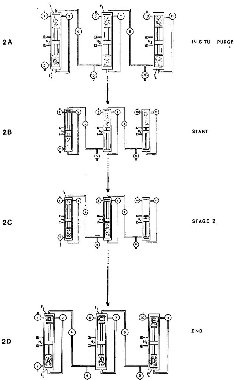
**Figure 2** A pictorial representation of four of the different stage of an *in situ* cascade ultrafiltration. The position of the pistons and the fractions A, A', B, C, D and E obtained are shown in 2D.
