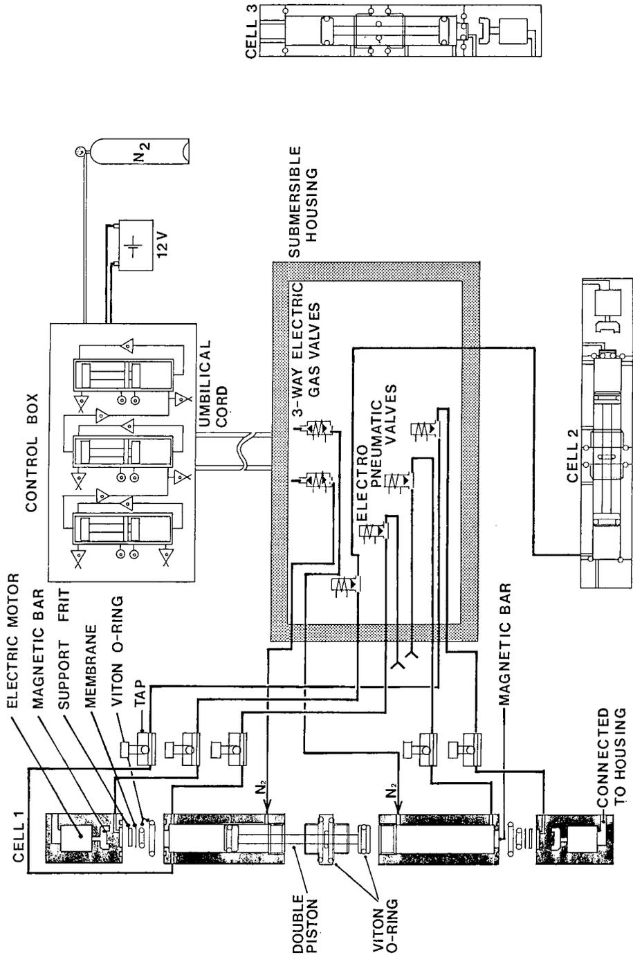
Figure 1 A schematic view of the *in situ* cascade ultrafiltration unit. On the left, an exploded view of an ultrafiltration cell.
